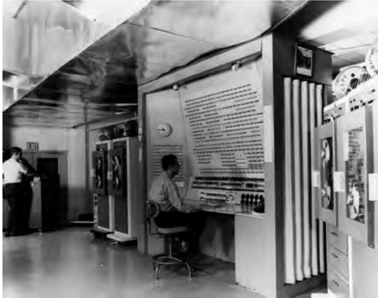
United States Army Ballistic Research Laboratories, Console BRLESC, Ballistic Research Laboratories Electronic Scientific Computer. Courtesy of the U.S. Army Research Laboratory.
